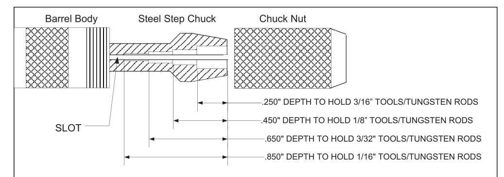
Holds fractional size drills, tools and tungsten rods with 1/16", 3/32", 1/8" and 3/16" diameter shanks
